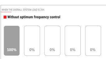
Since the compressors are running at inefficient frequencies, the efficiency of the whole system is lower.
