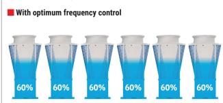
Our modules are equipped with inverter compressors, so the system can be operated in frequency ranges in which the efficiency of each module is at its peak. Optimum frequency control of each unit increases the efficiency of the whole system.
