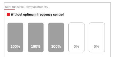
With non-inverter compressors, it is only possible to turn the unit on or off, and the compressor frequency cannot be adjusted according to the required capacity.
